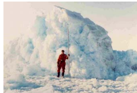
view of a “crushed ice extrusion remnant in the caisson’s wake
